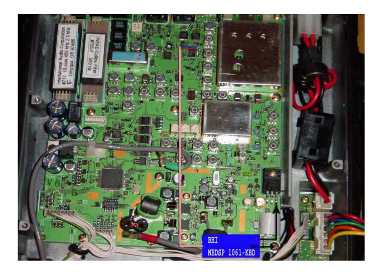
The upgrade using the DSP module involves the removal of small surface mount component, soldering of wires at the SMT level, and the drilling holes in the transceiver cover. Be certain you have the skill and all the tools required to perform it.
