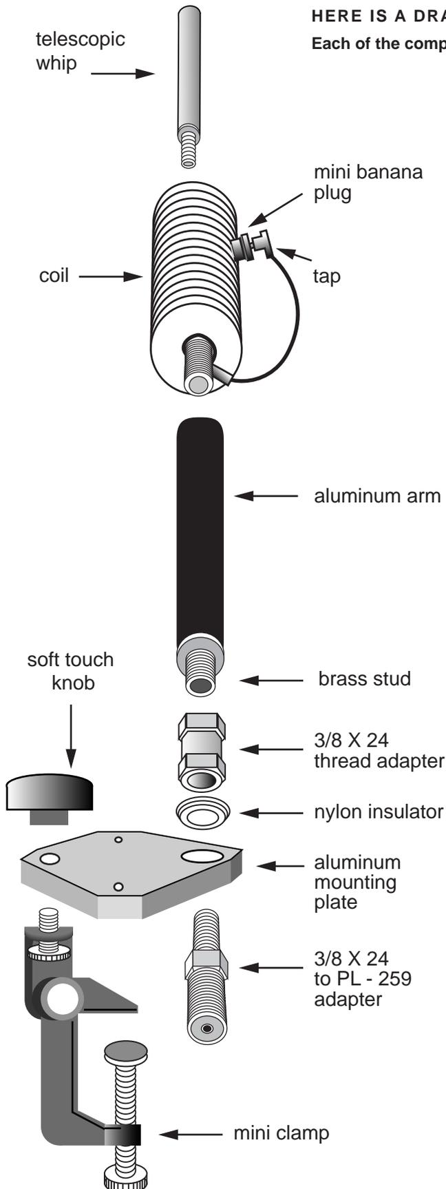
This antenna came about as a part of the **modular Buddi-pole system**. One of the dipole arms was designed to be mounted vertically, so that if one wanted to change from a horizontal to a vertical without purchasing a second antenna, this would be a solution.
