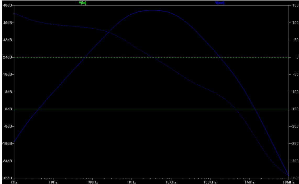
*Now, that's audio...over 40dB gain from 500Hz to 22kHz*
