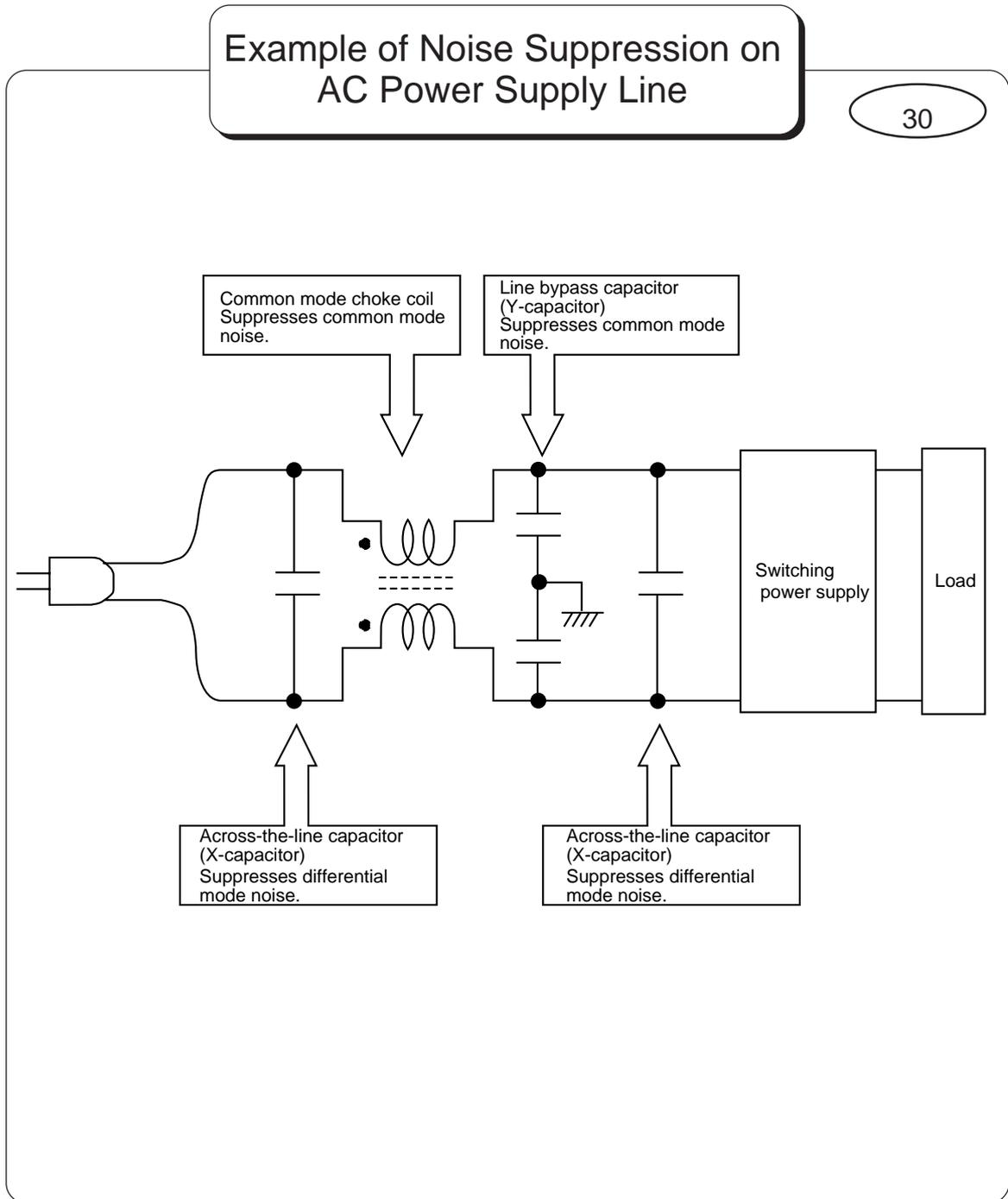
The above drawing shows an example of noise suppression on an AC power supply line.
