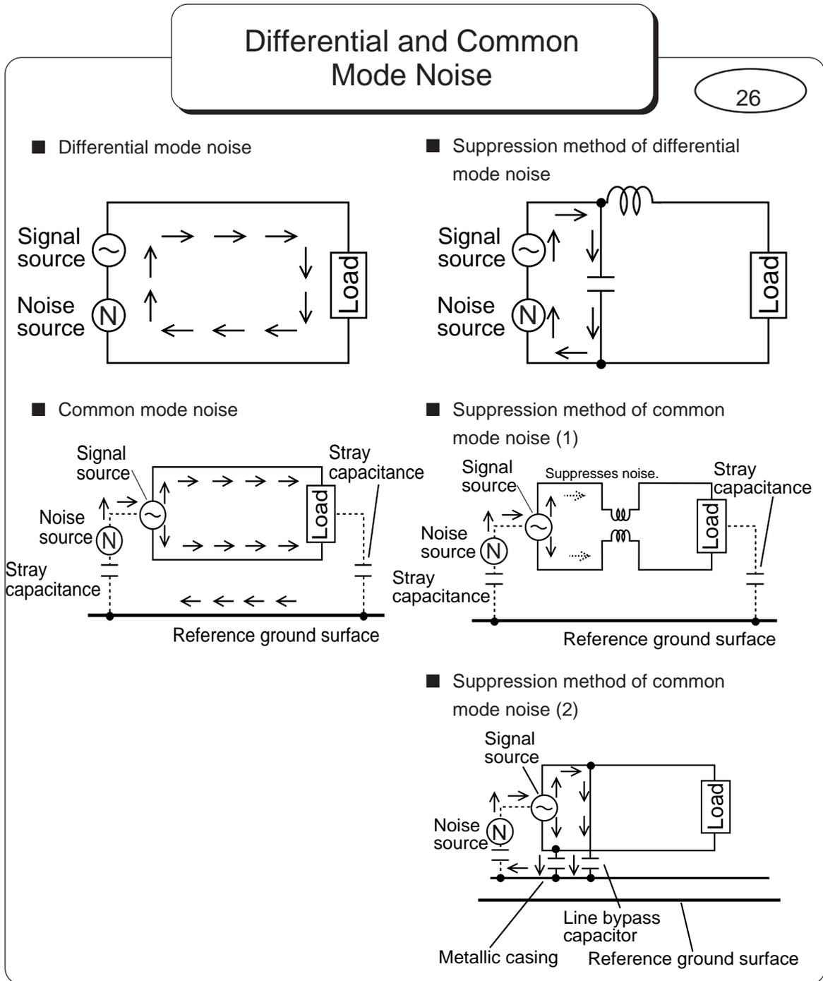
Noise is classified into two types according to the conduction mode.
