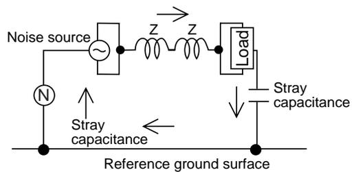
Common mode choke coils are used to suppress common mode noise. This type of coil is produced by winding the signal or supply wires one ferrite core.
