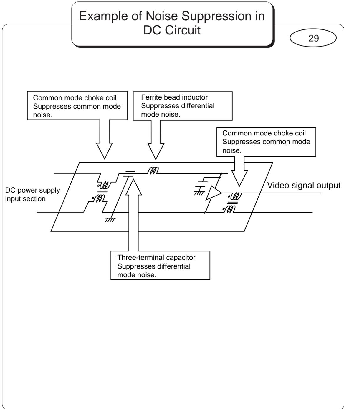
The above drawing shows an example of noise suppression in the DC circuit.
