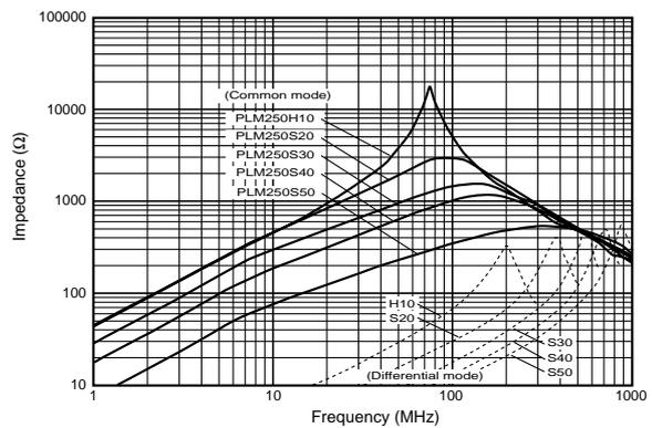
Since magnetic flux cancels out inside the ferrite core, impedance is not produced for differential mode current. The magnetic saturation problem is small. Common mode choke coils are suited for common mode noise suppression on lines with large current flow, such as AC/DC power supply lines. Since they do not affect signal waveform, they are also suited for common mode noise suppression on lines where signal waveform distortion causes a problem, such as video signal lines.
