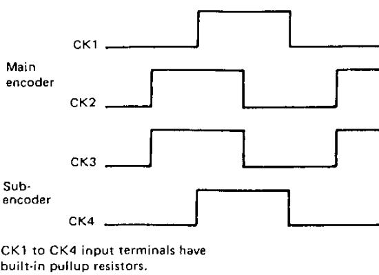
Fig. 16 Waveforms of IC26, CK1 to CK4,
