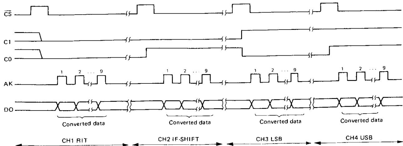
Fig. 25 A/D converter data read timing chart
