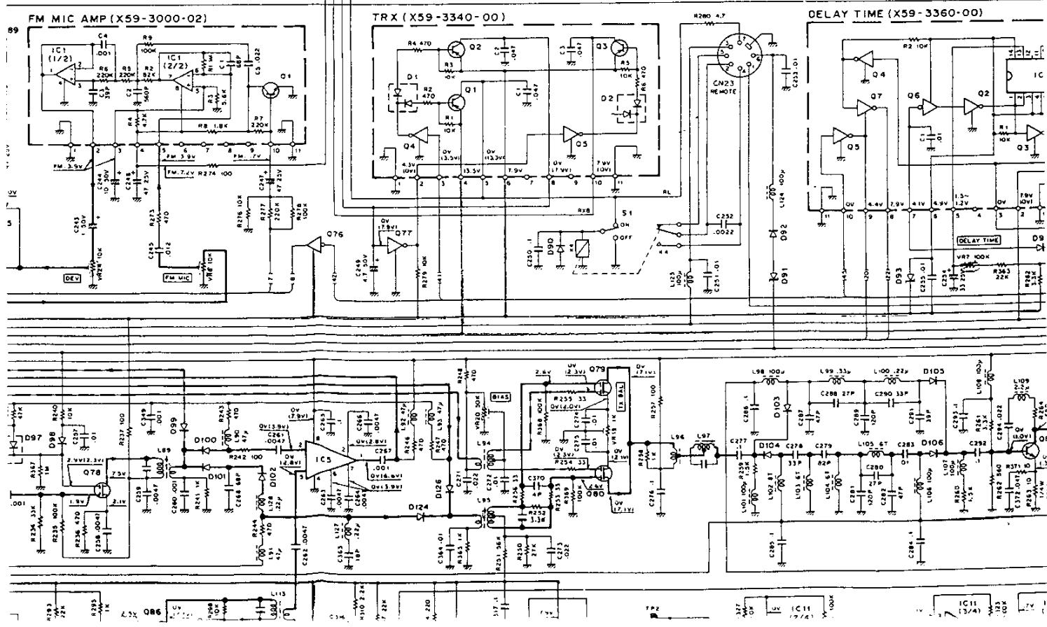
Voltage measurement condition f = 14MHz, Mode : USB. ( ) : TX.
