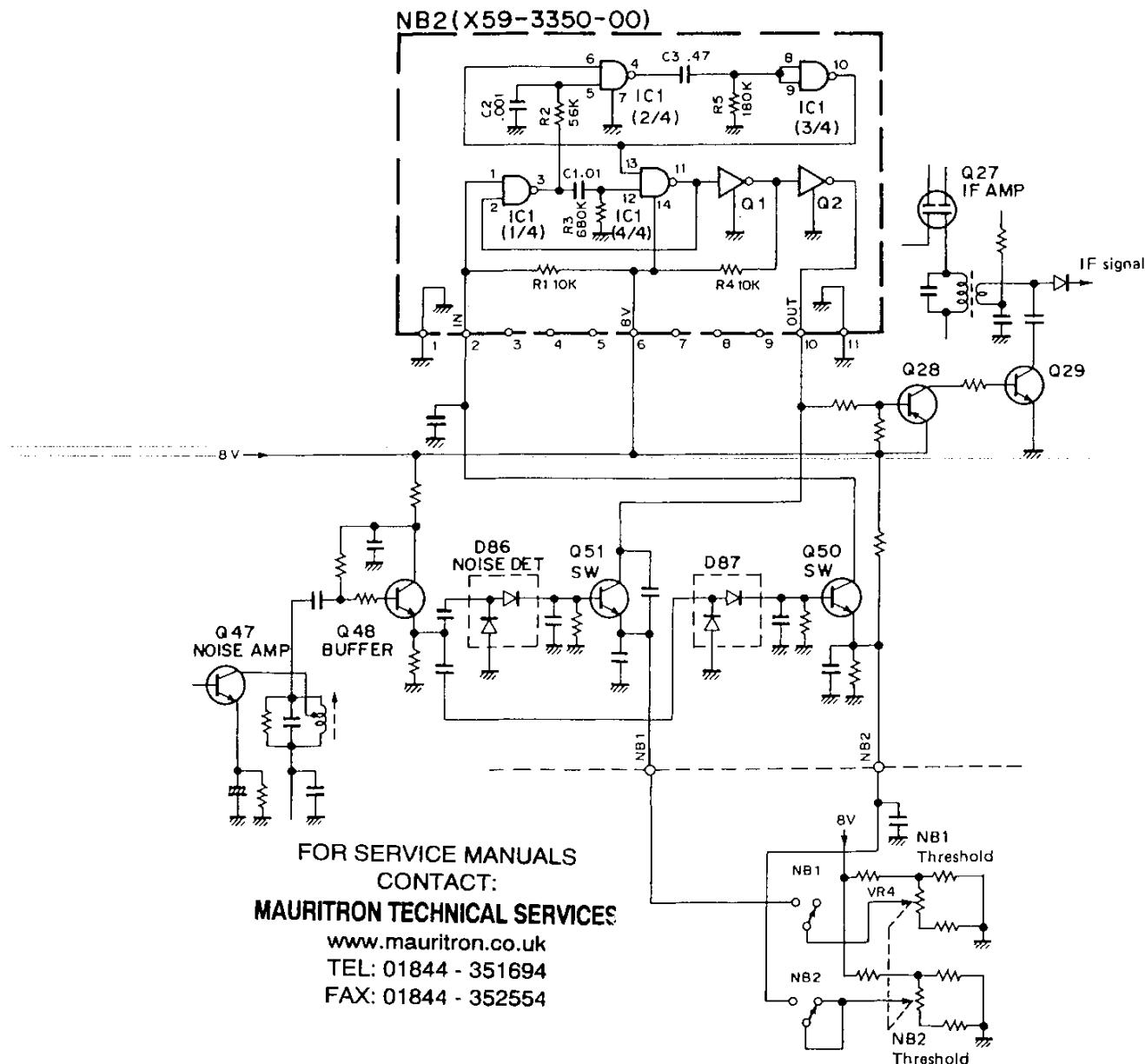
Fig. 4 Noise blunker circuit
