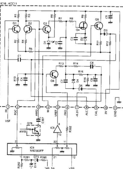
Fig. 10 ALC, Power control, SWR protection circuits
