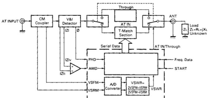
Fig. 16 AT control block diagram
