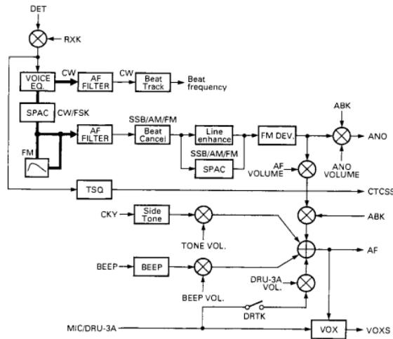
Fig. 19 DSP function block diagram (RX)
