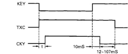
Fig. 12 Transmit/receive signal timing chart
