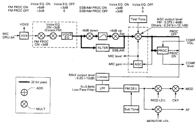
Fig. 18 DSP function block diagram (TX)
