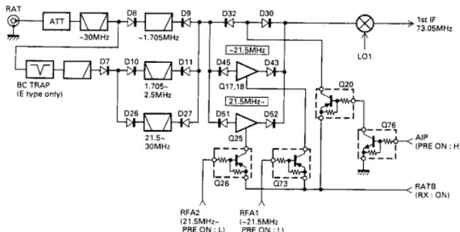
Fig. 6 Receiver front-end block diagram
