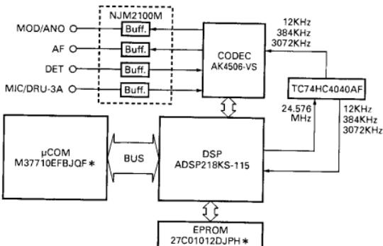
**Fig. 17** DSP section block diagram
