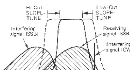
Fig. 9-E SSB-slope tune
