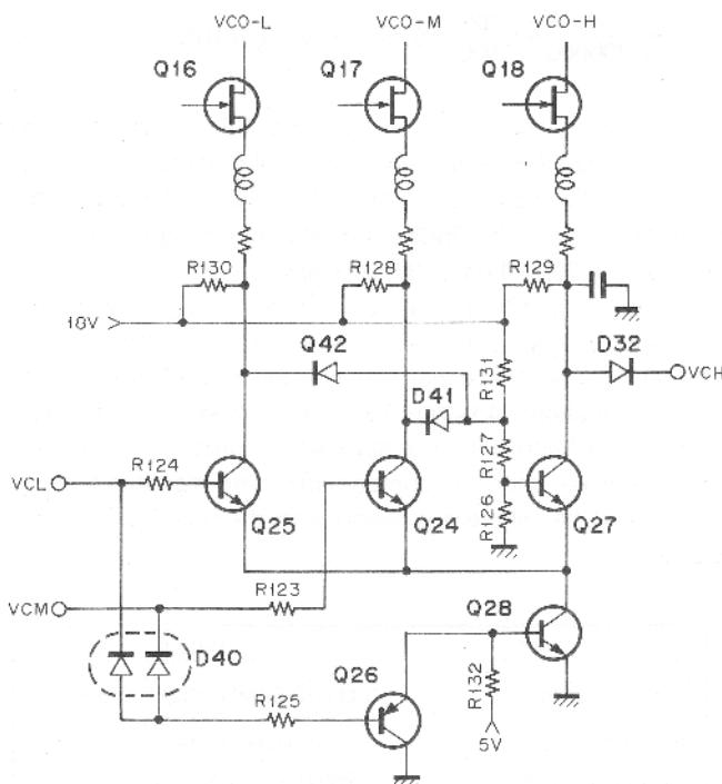
Fig. 4 VCO selector circuit
