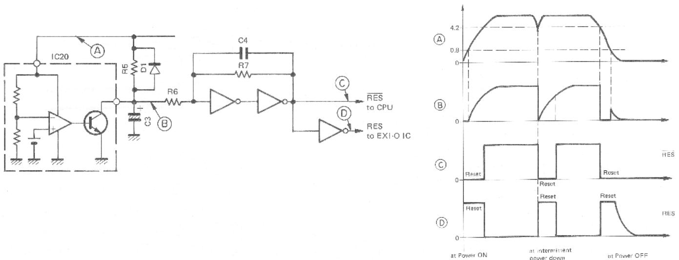
Fig. 32 Reset circuit
