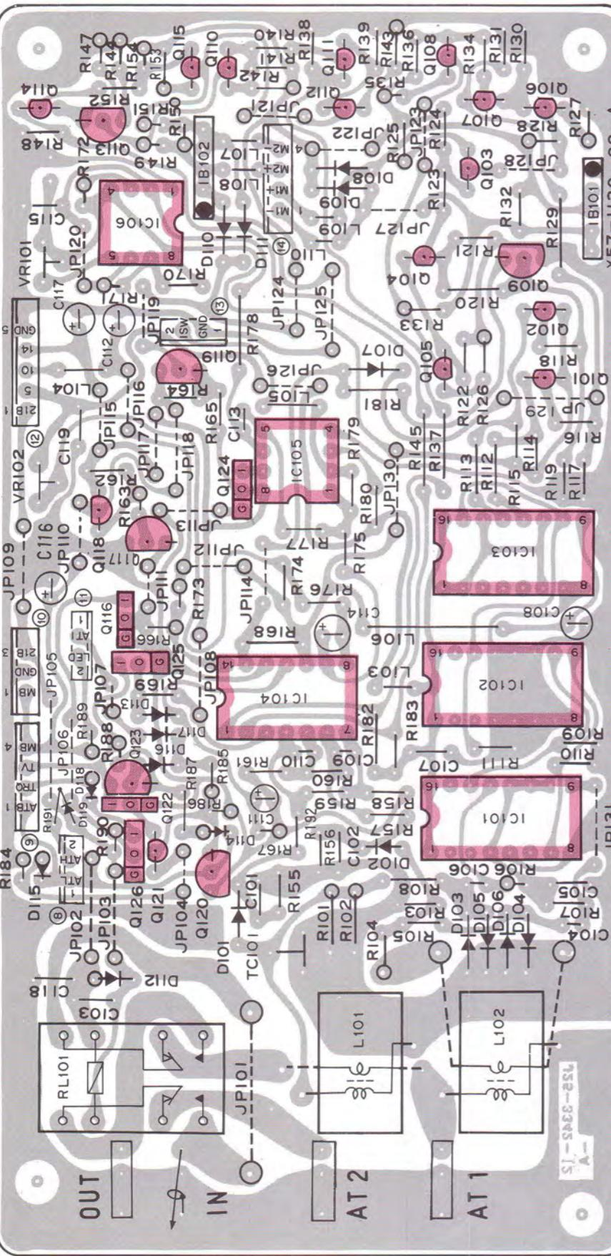
AT UNIT (B) (X57-1130-00) Component side view
