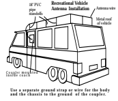
Use a separate ground strap or wire for the body and the chassis to the ground of the coupler.
