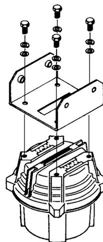
2. Insert the elevation rotator into the U-bracket, then fasten the elevation rotator using four M8x25 bolts, spring washers and flat washers.
