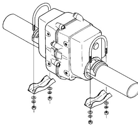
Be sure to leave enough slack in both the elevation control cable and the coaxial cable feedline around the azimuth rotator so the antenna can rotate 450° without straining the cable or feedline.
