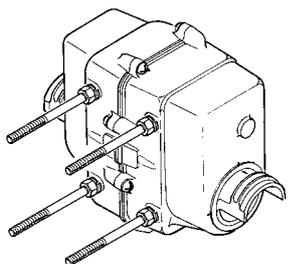
2. Slip an 8 mm flat washer over each installed stud bolt, and then the pipe clamps. Place another flat washer and then a spring washer over the end of each stud bolt, and start a nut on each to hold the hardware in place.
